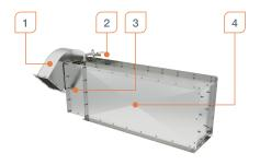
The point filter consists of the following main components, the dust air chamber [4], the clean air chamber [3] and the fan [1]. The point filter is cleaned using compressed air supplied via the central compressed air connection [2] and controlled via the filter control unit.
