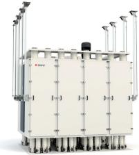
The plansifter is a sorting machine which separates the product from various roller mills or other grinders. It moves circularly in a horizontal plane. The product always flows from top to bottom, from one sieve to another, on the path called sieve channel. Drizzling from top to bottom, only a part of product passes through the sieves, the rest remains on the screen cloth.
