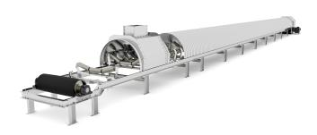
**Technical data** RBC800H RBC1000H RBC1200H RBC1400H Capacity (Bulk density Weight 400 t/h 600 t/h 800 t/h 1000 t/h 750 kg/m³) weight 1333 m<sup>3</sup>/h Volume 533 m³/h 800 m<sup>3</sup>/h 1067 m<sup>3</sup>/h Belt speed Nominal 2.5 m/s Drive unit Double right angle gearmotor with backstop Sound pressure level Up to 77 dB(A) Operating conditions -15°C to +40°C ambient
